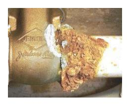
Galvanic Corrosion - Another example of the higher corrosion activity usually existing at direct brass to black iron connections.
